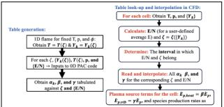
**Fig. 1.** Schematic of the manifold generation of 2D plasma energy fractions and their utilization in the phenomenological model.
